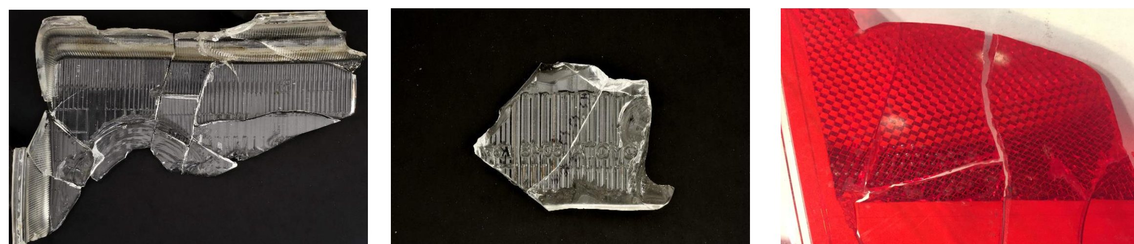
From left to right: Glass vehicular front headlamp, glass vehicular front headlamp, plastic vehicular taillight. All are exemplar physical matches.
